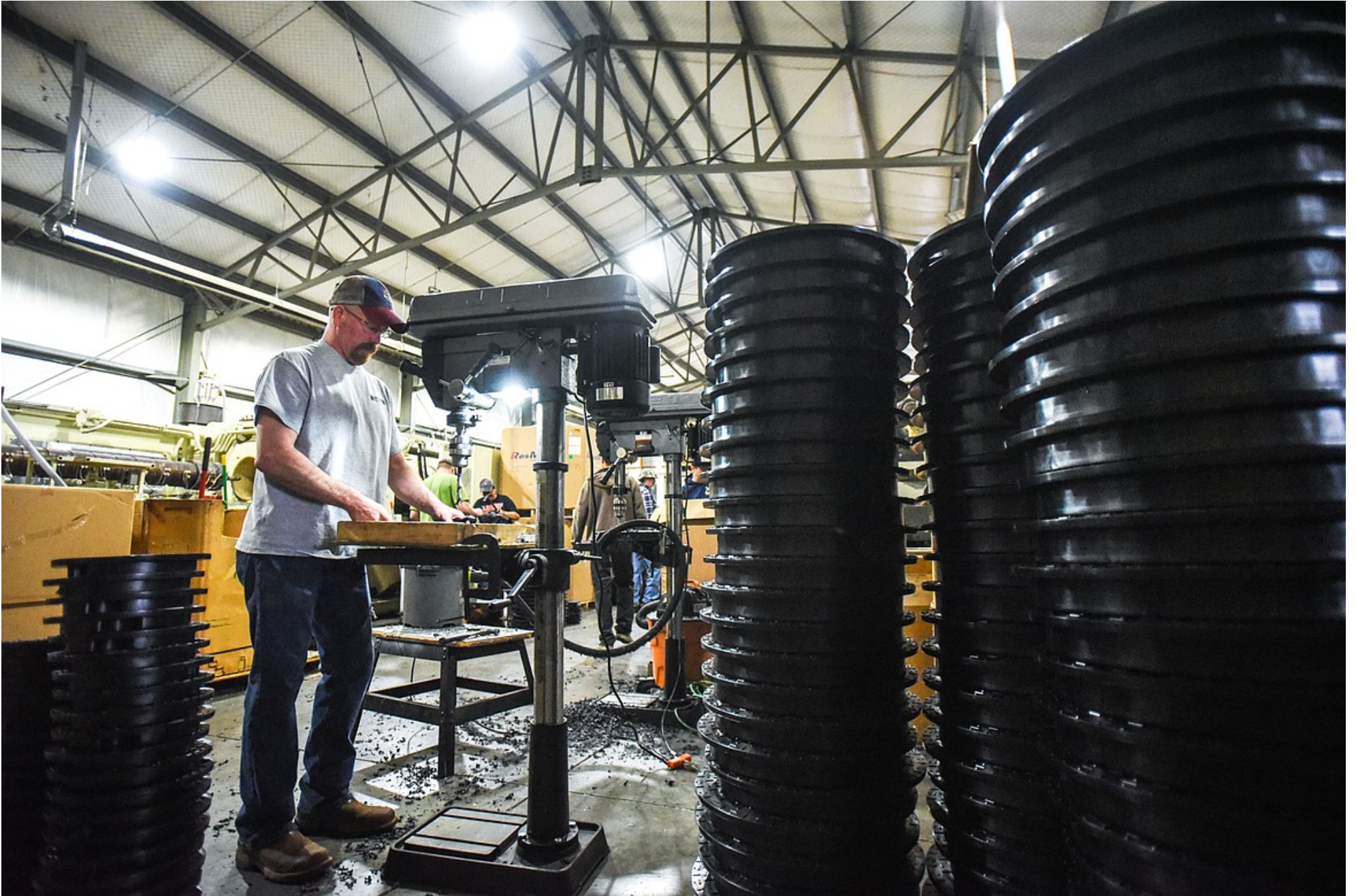
Bill Cook works on repositioning the locking mechanism on injection molded water meter lids at Northern Plastics on Wednesday, May 19. (Casey Kreider/Daily Inter Lake)
